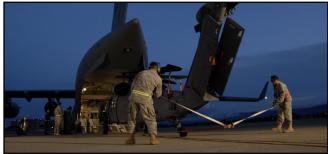
(U.S. Air Force photo by Tech. Sgt. Ray Aquino) 129th Maintenance Group personnel direct an HH-60G Pave Hawk rescue helicopter into a C-17 Globemaster, May 3.
